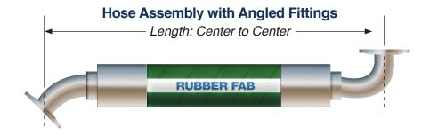
When figuring out the angle needed of an elbow we suggest you follow these simple directions. Assume that the hose fitting #1 is in your hand at 0°. When selecting a hose with multiple angled fittings, simply let us know where fitting #2 should be facing.
